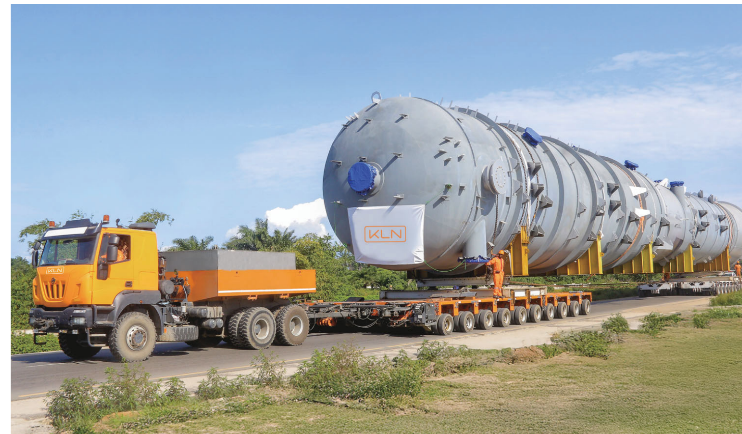
KLN Group delivered a large-scale fertiliser plant, including an ammonia converter weighing up to 643.50 tonnes, from South Korea to Nigeria via road freight between May and July 2025
